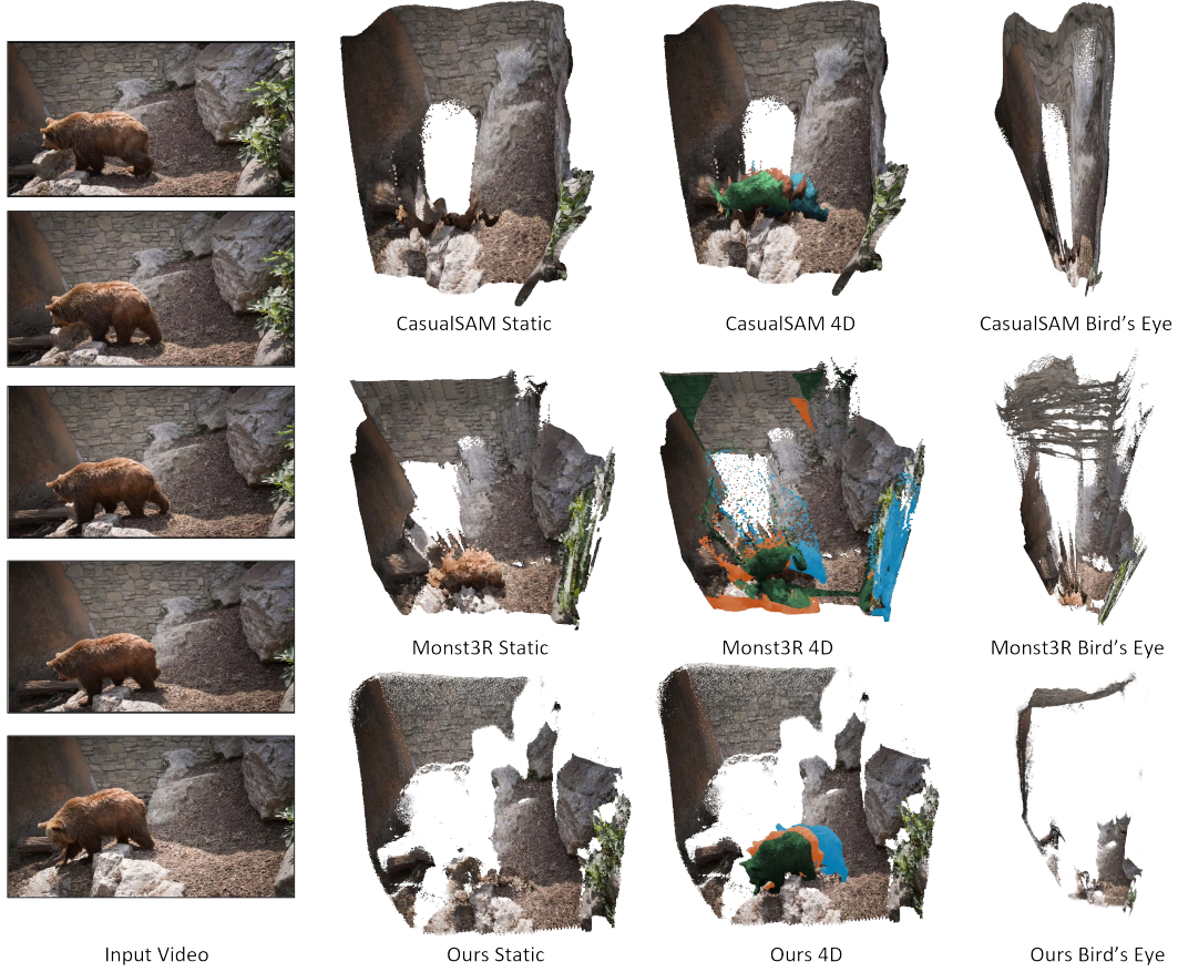
Figure 4. Qualitative results of 4D reconstruction on the DAVIS [43] dataset. CasualSAM [68] suffers from slanted geometry, and Monst3R [65] has unclear geometry and does not resolve conflicts from multiple views (note the wall in the bird’s-eye view). Both CasualSAM and Monst3R lack clean dynamic reconstruction and segmentation. Uni4D achieves a realistic layout, thanks to joint optimization, and provides accurate dynamic segmentation and reconstruction by leveraging foundation visual models as cues.
