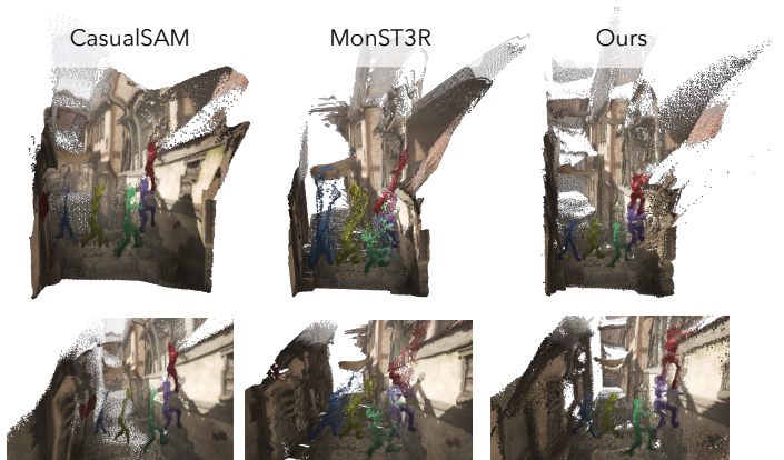
Figure 7. Qualitative results of 4D reconstruction on Sintel dataset. We highlight and contrast performance on (1) dynamic objects and (2) geometry on planar surfaces.
