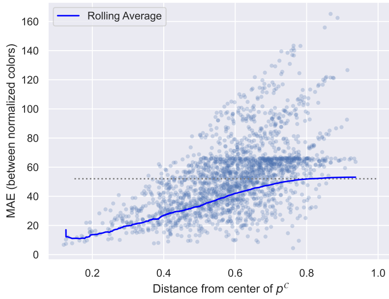
Figure 16: Accuracy of the predicted RGB values (normalized by alpha) as a function of the distance between the analyzed sample from the center of the calibration set distribution.
