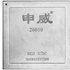
(k) 128-core Sunway SW26010 [LFF + 18]
