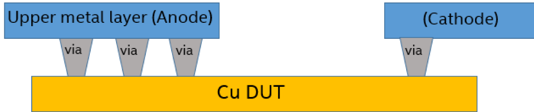
Figure 3.2. EM DUT configuration, current from CMOS circuit arrives at anode and flowing to cathode.
