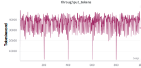
Figure 9. The training throughput of GaLore-type low-rank optimizer with many spikes due to the expensive SVD operation every 200 steps.
