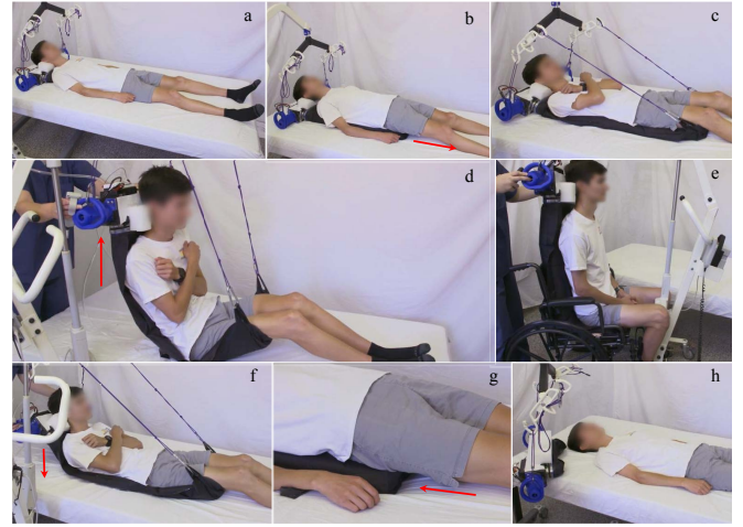
Fig. 5: Patient transfer demonstrations. (a-b) With the soft growing robotic sling system placed under the participant's head, the robotic sling grows underneath the participant's body. (c-d) Participant is lifted from the bed with the deflated robotic sling using a Hoyer lift. (e) Hoyer lift is maneuvered by the caregiver to transfer the participant to a chair. (f) Participant is transferred back to lay in the bed. (g) Robotic sling automatically retracts itself from under the participant. (h) The system, including the wide base, is manually removed from under the participant's head.
