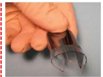
1μm-thick Si membrane encapsulated in a Hybridsil® thin film
