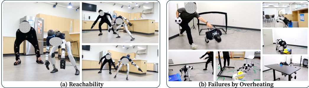
Figure 8: (a) Extreme reachability by TWIST. (b) Failures caused by motor overheating.
