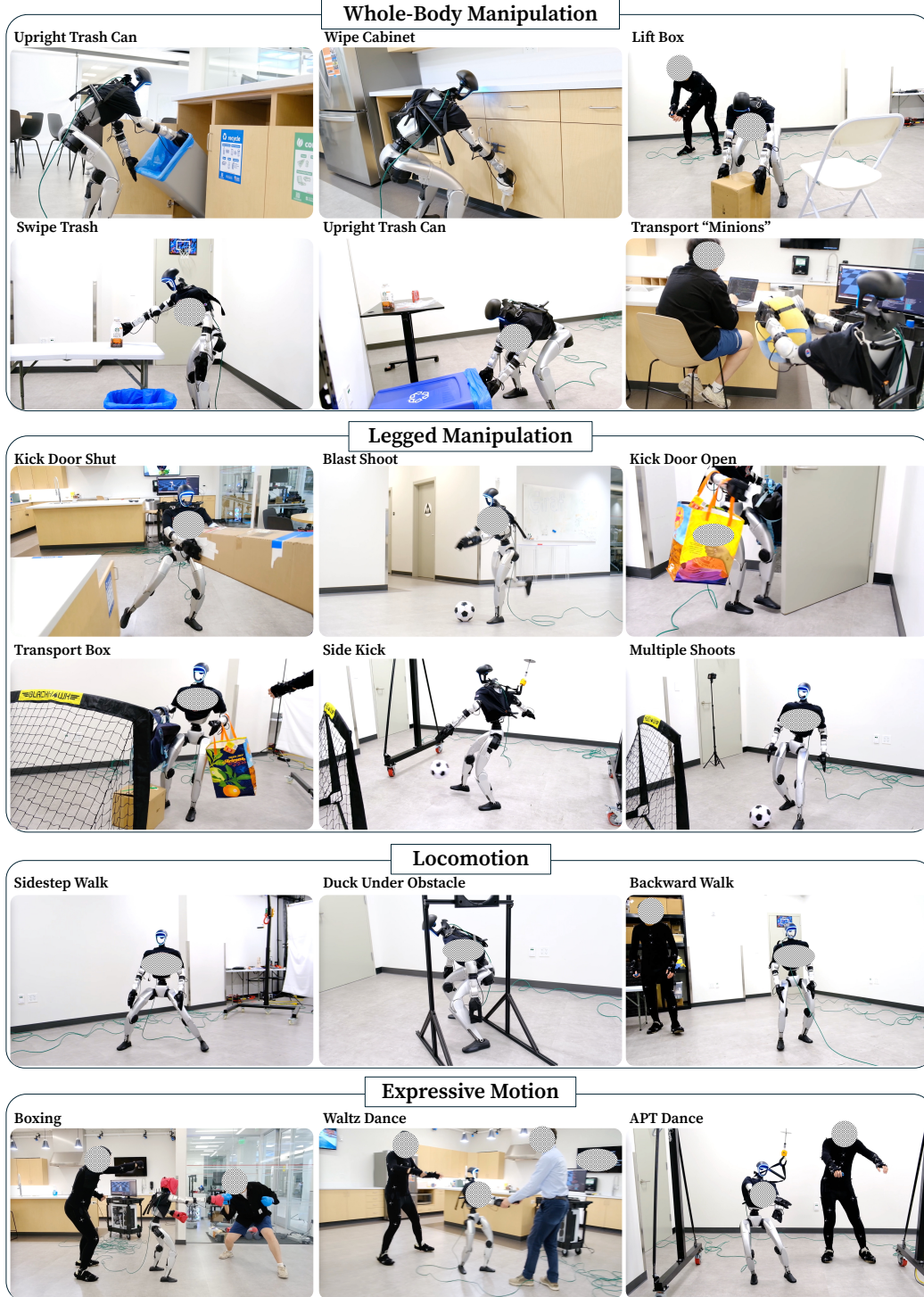
Figure 1: Our Teleoperated Whole-Body Imitation System (TWIST) presents versatile, coordinated, and human-like whole-body skills on real-world humanoid robots. Our robot can perform whole-body manipulation (e.g., lifting boxes from the ground), legged manipulation (e.g., kicking the football), locomotion (e.g., ducking under the obstacle and walking backwards), and expressive motions (e.g., Waltz dance).
