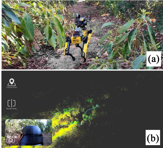
Fig. 7: (a) Snapshot shown the robot traversing rough terrains in AES fields at UC Riverside while carrying a heavy payload. (b) LiDAR-based mapping and localization assisting with teleoperation.
