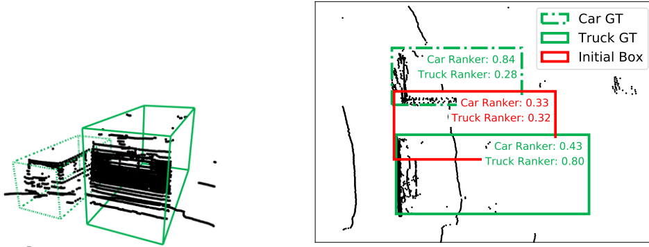
(a) Real example of a scenario where two objects with different categories ('car' and 'truck') are close. (b) Visualization of two class-specific rankers ( i.e. , car ranker and truck ranker). Each ranker assigns different scores to different bounding boxes but predicts the highest score for the desired class.
