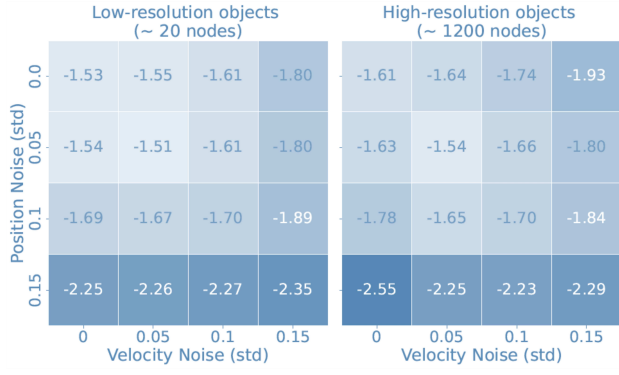
Fig. 5. Performance under varying levels of synthetic noise and object resolutions in the deformable task, showing GRPD’s resilience to perturbations and ability to handle high-resolution inputs.
