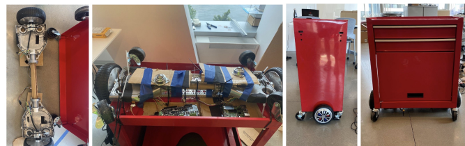
Fig. 2. We built Prototype 1 by connecting the Garbatrage hoverboard circuit [63] to a tool cart using metal chassis, cardboard, and tape.
