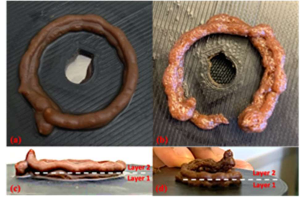
Fig. 3. (a) Overhead view of the complete circle design printed in ambient pressure; (b) overhead view of the complete circle design printed in vacuum chamber pressure; (c) side view of complete circle design in ambient pressure displaying distinct printed layers; (d) side view of complete circle design in the vacuum chamber pressure displaying distinct printed layers.
