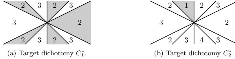
Figure 2: Illustration of Example 2.3. For a given set of input data points the figure shows the polyhedral fan \Sigma_{\mathcal{D}} in parameter space along with the value of the 0/1-loss for the two target dichotomies C_1^* (left) and C_2^* (right). The sets of minimizers are shown in gray.
