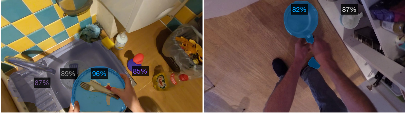
Figure 11. Additional detection results from prompting the Detic [52] CLIP-based detector with our audio embeddings of natural impact sounds from egocentric videos from kitchens [7]. (Left) From the sound of setting the red-handled knife on the plate, the detector successfully predicts the correct plate (highlighted blue, bottom center) with high confidence. It also predicts the other plate, sink, and body of the hands soap dispenser with relatively high confidences, but ignores other objects. (Right) As a failure case, from the sound of the metal pan stacking onto the metal pot below it, the detector predicts the ceramic bowl in the cabinet (highlighted gray at upper right of the image) with highest confidence. It also predicts the correct metal pan (highlighted blue, upper center) with relatively high confidence.
