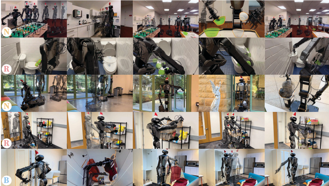
Figure 1: Everyday household activities enabled by BEHAVIOR ROBOT SUITE (BRS), showcasing its three core capabilities: bimanual coordination ( B ), stable and accurate navigation ( N ), and extensive end-effector reachability ( R ).
