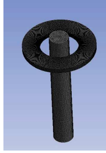
Figure 4.2 Ansys AQWA model for calculation of hydrodynamic coefficients
