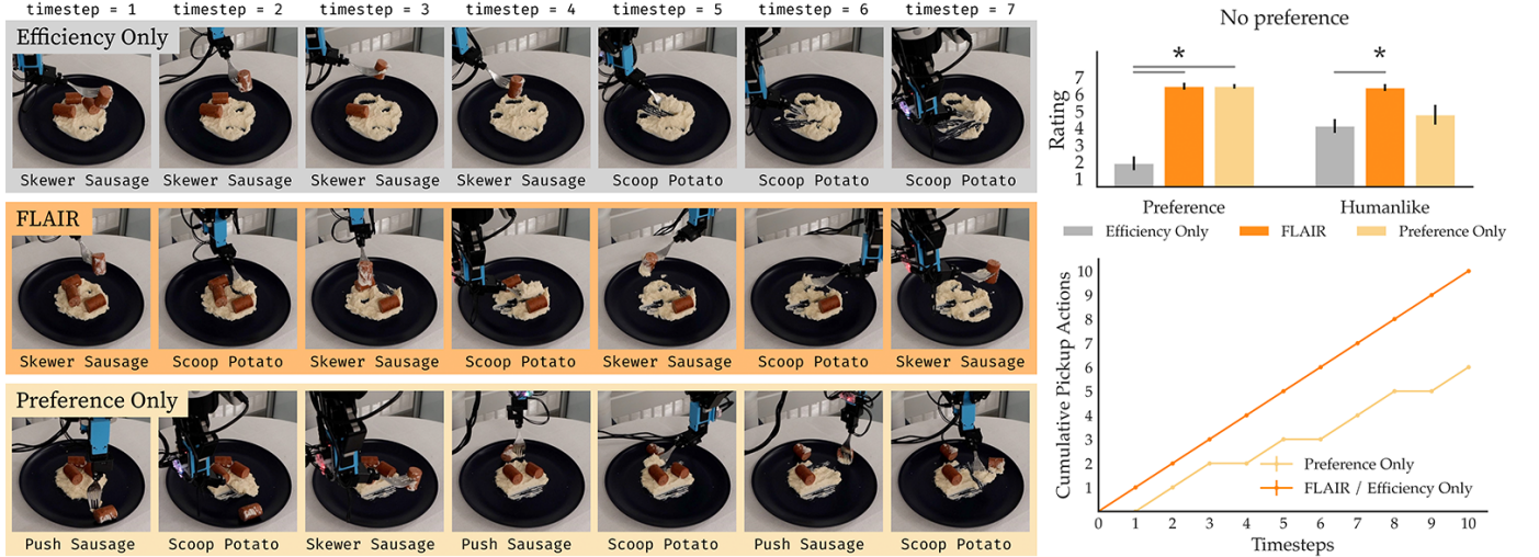
Fig. 5: Example run on a plate with mashed potatoes and sausages where the user specified no preference. FLAIR, which balances user preferences (bite variety) and efficiency, is judged by users to better adhere to preferences than Efficiency-Only and outperforms Preference-Only (Commonsense-Only) in plate clearance. Consequently, FLAIR is considered to provide a more human-like feeding experience compared to the baseline methods. Note that * indicates statistical significance ( p -value < 0.05 ), determined via a Mann-Whitney U test.
