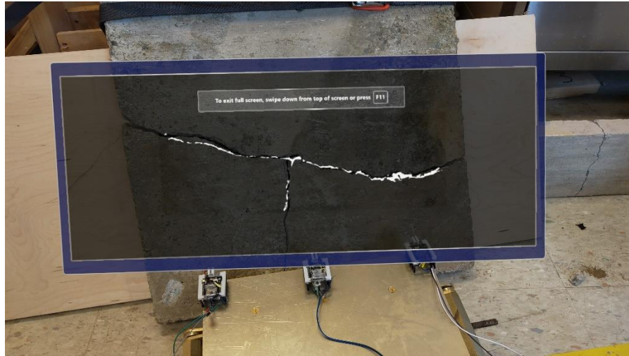
Figure 7 Crack identified by multi-view imaging with swarm robot. Segmented and merged crack image displayed on inset with augmented reality interface [7].
