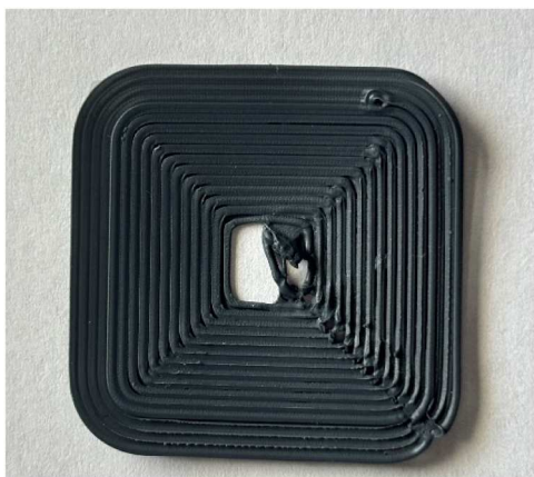
Fig. 13. 3D printed sample of pure Walmart Bag filament.
