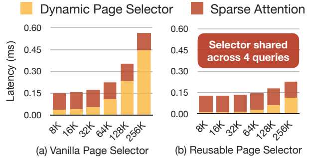
Figure 14: Effect of Reusable Page Selection. The overhead of the dynamic page selector is significant, as its complexity increases linearly with input sequence length. Our Reusable Page Selection effectively mitigates this issue. The latency breakdown is evaluated on Llama-3-8B.
