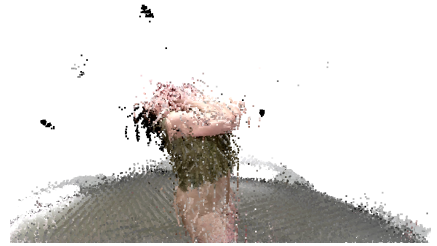
FIG. A.1. Block artifacts arising from unscaled depth encoding when we use naive H.265 YUV 16-bit variant.
