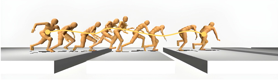
Figure 1. Visual whole-body control for humanoids. We present Puppeteer, a hierarchical world model for humanoid control with visual observations. Our method produces natural and human-like motions without any reward design or skill primitives, and traverses challenging terrain.
