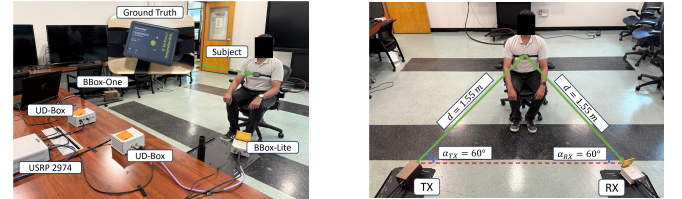
Figure 3. Breathing patterns detection setup. Left: All entities. Right: Specific antennas and subject setup for breathing pattern detection.
