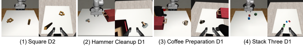
Figure 5: A subset of experimental environments from MimicGen. Left: external view of the task. Right: eye-in-hand observation used in the experiments. The full set of tasks is shown in Appendix D.
