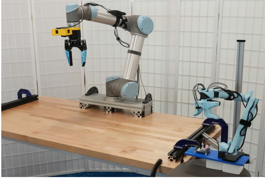
Figure 9: Real-world experimental setup. We use a UR5 robot equipped with a Robotiq-85 gripper and custom-designed soft fingers. A GoPro camera is mounted on the wrist to capture visual observations. Demonstrations are collected using the Gello teleoperation interface (bottom right).
