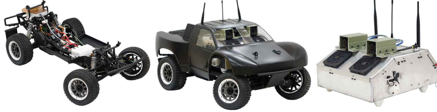
Fig. 14: AutoRally chassis and compute box [24].
