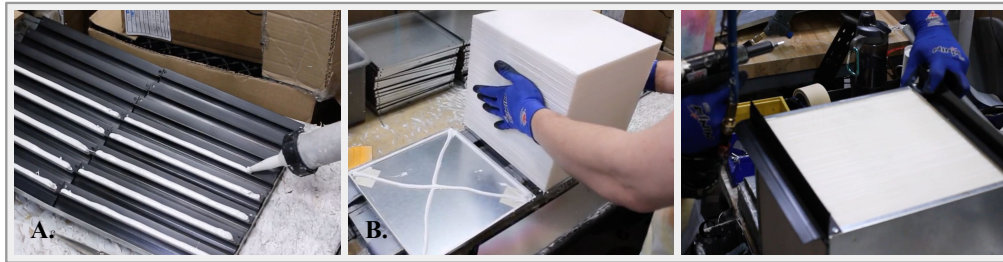
Figure 4.4: A subset of the steps involved in the manufacturer's assembly process. A. applying silicone to gaskets. B. applying silicone to pans and beginning the assembly process. C. continuing the assembly process by attaching gaskets.
