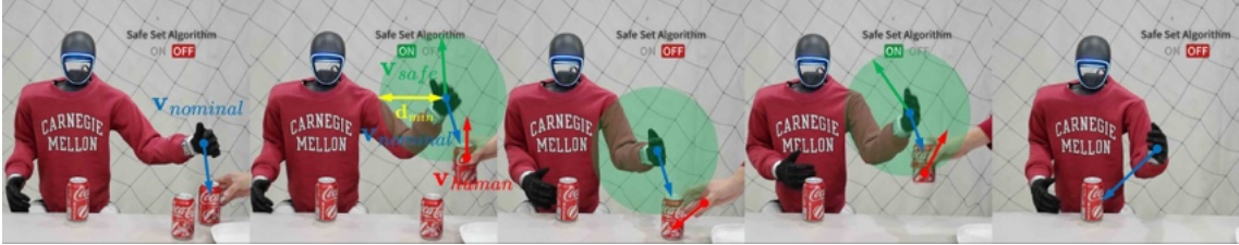
Fig. 7. 4.4 Limb-level collision avoidance with teleoperation commands.
