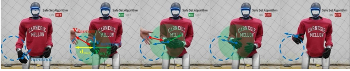
Fig. 6. 4.3 Limb-level collision avoidance with dynamic humanoid reference poses.
