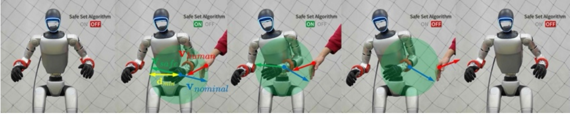
Fig. 5. 4.3 Limb-level collision avoidance with static humanoid reference pose.
