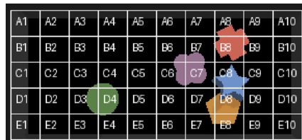
Figure 7: The Region-Based Placement Tool overlays the workspace with a labeled grid, allowing the VLM to reference specific spatial locations when issuing placement commands.
