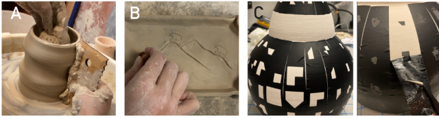
Figure 2: Ceramic tools. A) A rib can form the overall shape of the vessel while throwing. B) Bear-shapes. C) Stencil mask to selectively apply a decorative effect with underglaze [86].
