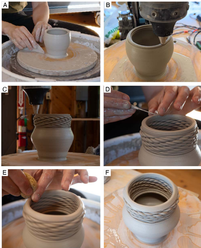
Figure 18: The workflow for transitioning between printing and throwing using the Wheelbot. A) An operator throws a vessel on a bat using a traditional pottery wheel. B) The operator mounts the bat on the XY stage of the Wheelbot using the pre-drilled screw mounts. It is automatically centered on the stage. The operator adjusts the Wheelbot's radius until the extruder is over the pot lip, then begins printing. C) The operator prints their desired form using the Wheelbot Mixer. D) If desired, the operator can return the printed form to the wheel for further manual modification. Here, they trim off the uneven top of the coil left by the printing process, and E) smooth and reshape the printed lip with a sponge. F) The completed pot.
