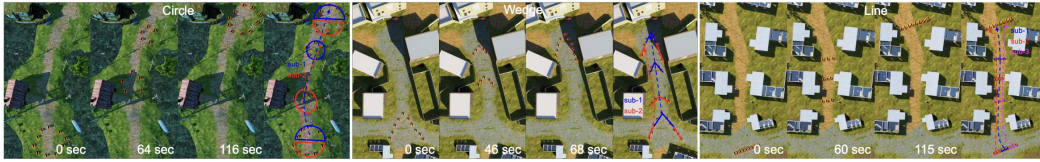
Figure 5: Qualitative results from Unity3D simulations in ROS1 using varying numbers of differential-drive Warthog robots in three formations while navigating a long, unstructured field environment.
