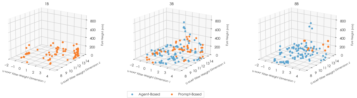
Fig. 4: A U-MAP projection of the design space explored by the two schemes. When using the 8B model, the Prompt-Based scheme suggested very similar parameter ranges numerous times. On the other hand, the Agent-Based approach was able to meaningfully explore the design space and improve eye height.
