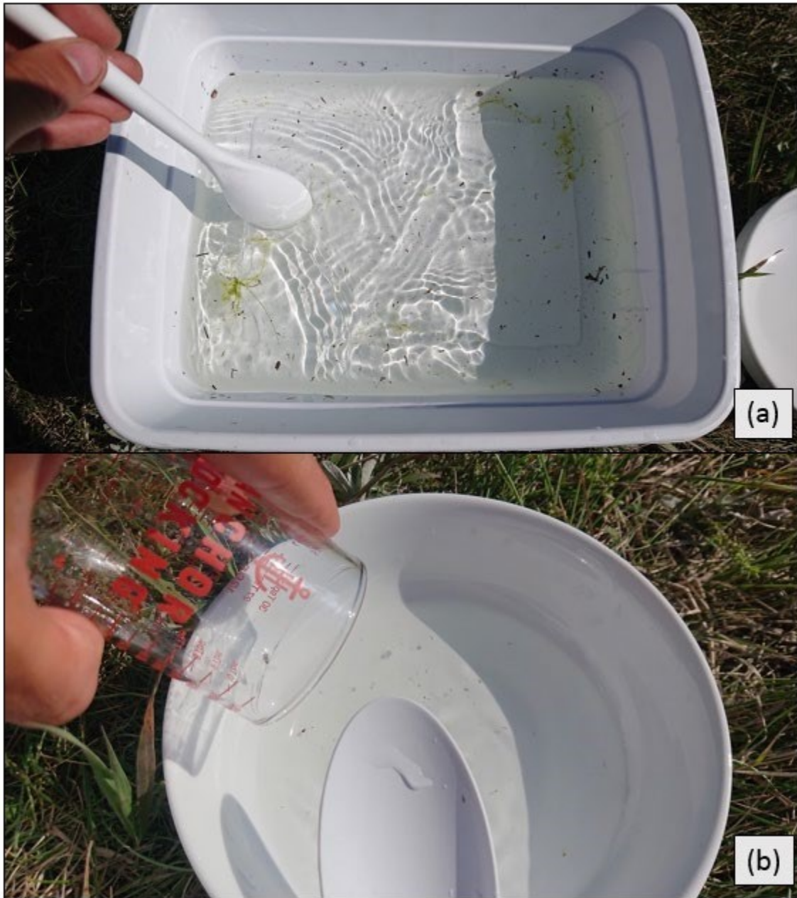
Figure S46: (a) The white plastic dish bin into which the net sweeps are rinsed when collecting a community sample. (b) a smaller white enamel bowl containing a subsample of Cladocera collected from an original sample in the white dish bin above.
