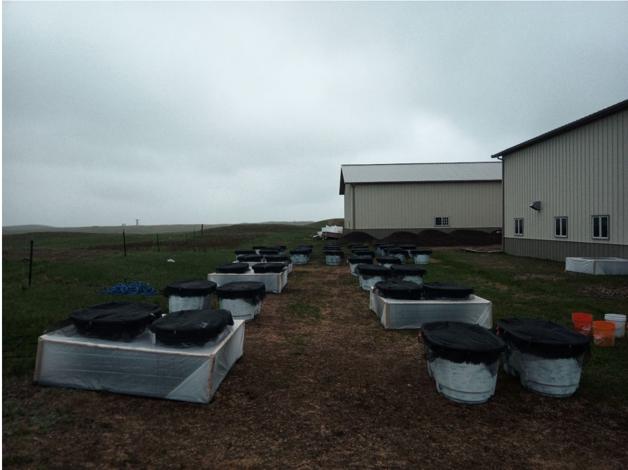
Figure S67: Physical arrangement of the array of mesocosms showing the pairs of mesocosms. The eight pairs in the foreground are those seeded with mixed sediment. Behind these is a second array of mesocosms for a separate experiment. Along the outer edges of that array are four additional mesocosms with local sediment. Each of those mesocosms is paired with the adjacent mesocosm in that array. These eight mesocosms, in total, make up the local sediment seeded mesocosms used in the current study.
