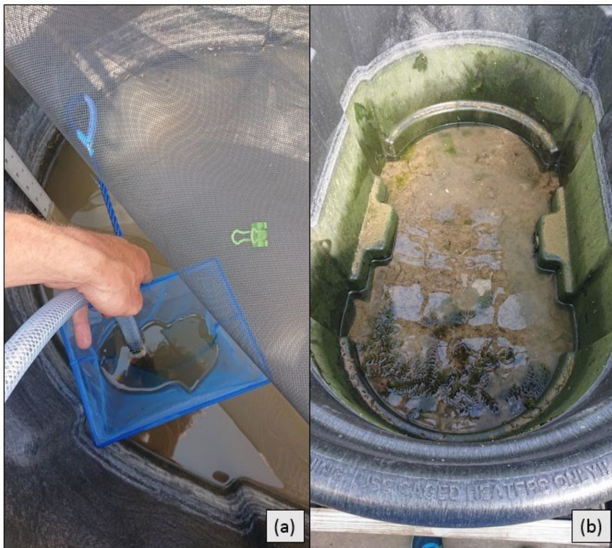
Figure S40: Pictures showing the process of draining the mesocosms during the drawdown. (a) The water is filtered through the net used for sampling and is drawn out using a transfer pump. (b) A mesocosm which has been drawn down to one inch of water remaining as specified in the drawdown treatment.
