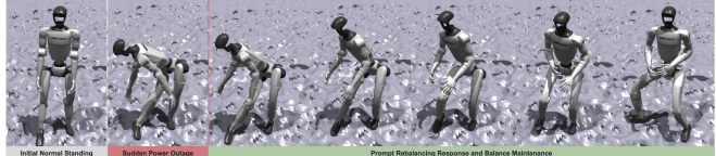
Fig. 7. Fall prevention when controllable. Under 0.5s of zero torque output (mimics a sudden power outage in real world), the robot rapidly initiates rebalancing response, allowing the robot to maintain stability, thereby preventing a fall. With stitching, robots are not necessary to fall every time it encounters imbalance situations.
