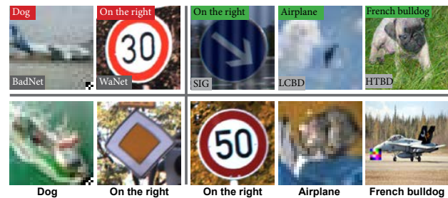
Figure 1. Illustration of dirty-label and clean-label attacks (Top row: poisoned training samples; Bottom row: backdoored test samples. Red: incorrect labels; Green: correct labels. Dirty-label poisoned samples always possess incorrect labels while clean-label poisoned samples are imperceptible compared to benign samples and possess correct labels.
