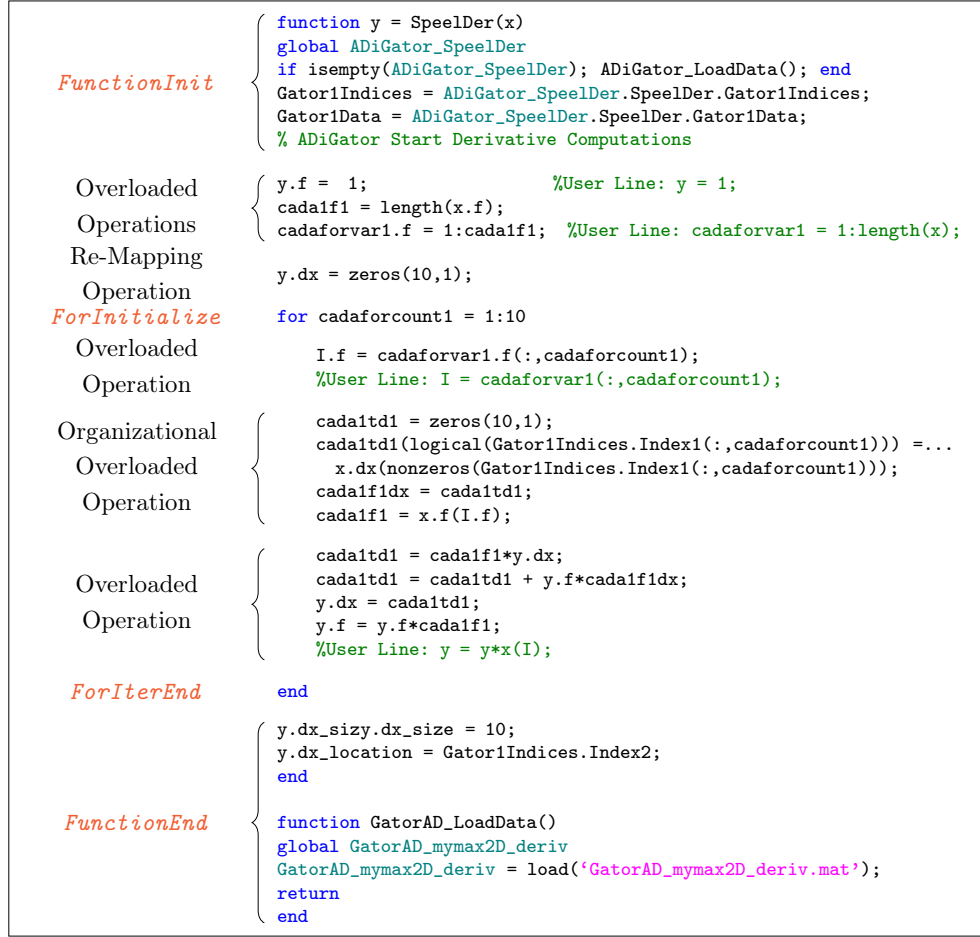
Fig. 14: Derivative Program for Speelpenning Problem for N = 10 Showing Origin of Each Printed Line of Code.
