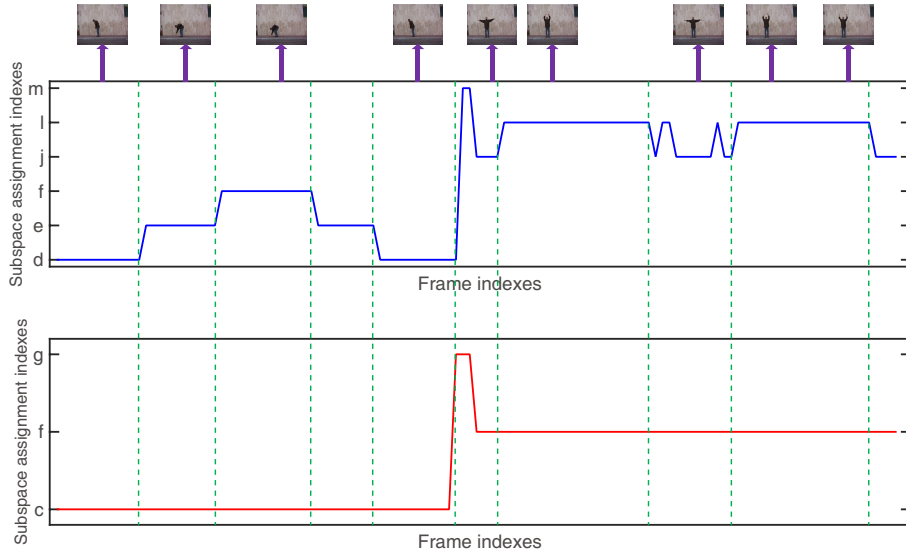
Figure 6. Subspace transition of a long sequence using subspaces at the 5th level (top) and the 3rd level (bottom). The subspace assignment indexes in the top/bottom figure correspond to the attributes in Fig. 5 and Fig. 4, respectively.
