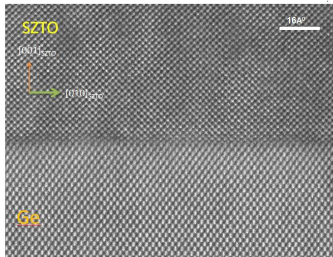
Figure 3. High angle annular dark field image of the SZTO-Ge interface for Zr content x = 0.7 .
