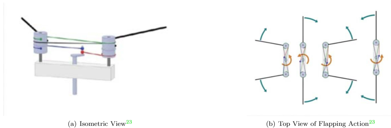
Figure 3. The AeroVironment Hummingbird Nano Air Vehicle Flapping Mechanism 23
