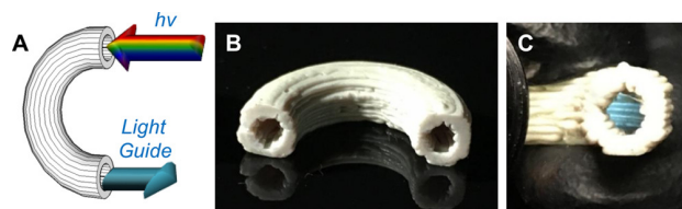
Figure 5. Model of object and concept of a polymer-based PC acting as a light guide (A). Photograph of the 3D-printed object with an outer diameter of 0.5 cm (B) that, when irradiated with a white flashlight from one opening, can guide green light to exit the other opening (C).
