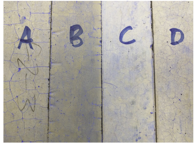
Fig. 6. Typical cracking patterns in (a) AAF concrete dried at early age, (b) AAF concrete dried after heat-curing, (c) AASC concrete dried at early age, and (d) AASC concrete dried after heat-curing.
