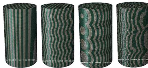
Fig. 3. Pillar models used with flat, cosine, arc segment, and FIB derived nanostructures (respectively from left to right). Al layers are depicted in green while SiC layers are depicted in gray. (For interpretation of the references to colour in this figure legend, the reader is referred to the web version of this article.)
