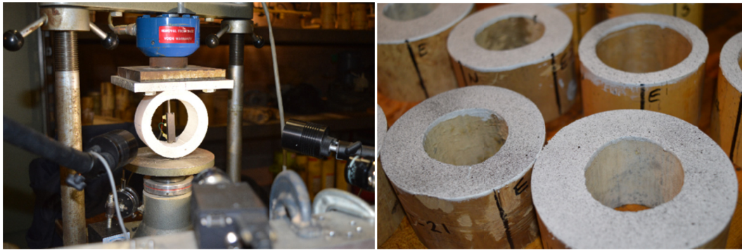
Fig 2. Compression edge bearing test, a. Test arrangement (one DIC camera is in foreground), b. Bamboo rings prepared for DIC measurement.
