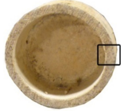
b) cross section of culm near node diaphragm
