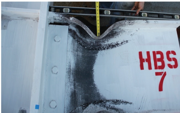
Fig. 18. Photograph showing post-test local flange buckling amplitude of HBS 7 (after one cycle of 6% drift).
