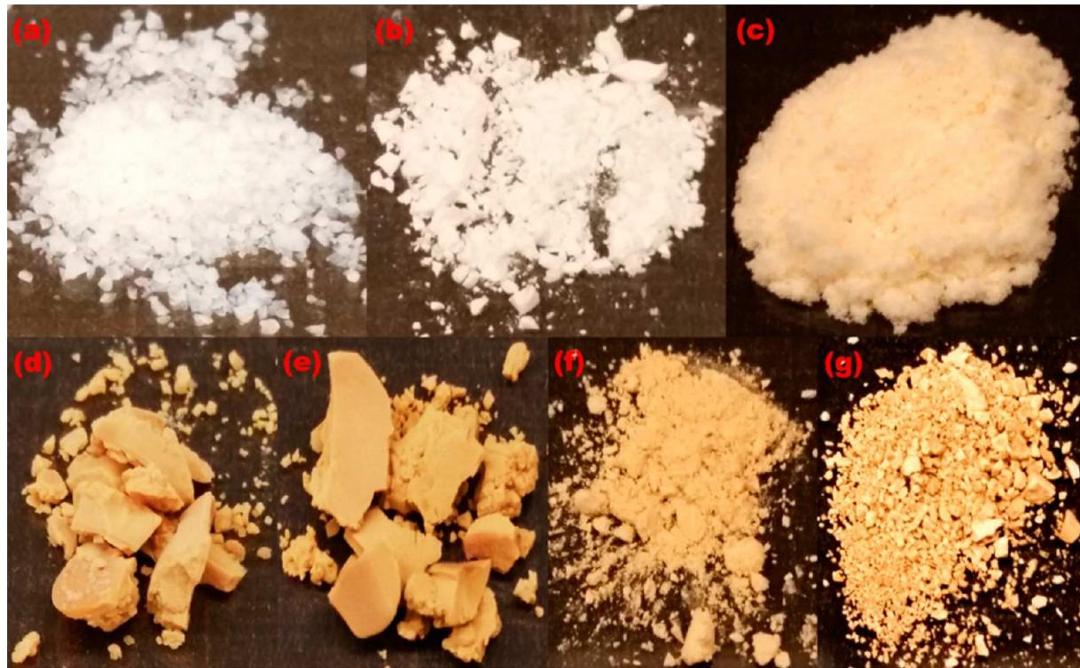
**Figure 1.** (a) ZIF-8 nanocrystals, (b) ZIF-8 microcrystals, (c) ZIF-8<sub>50</sub>–90<sub>50</sub> NSIC hybrid, (d) nano-ZIF-8–90 SALE hybrid made at 60 °C for 3 days, (e) nano-ZIF-8–90 SALE hybrid made at 90 °C for 8 h, (f) micro-ZIF-8–90 SALE hybrid made at 90 °C for 3 days, and (g) micro-ZIF-8–90 SALE hybrid made at 60 °C for 6 days. Each image occupies roughly 2.5 × 2.5 cm<sup>2</sup> area.
