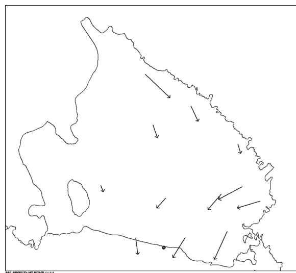
Figure 13. Twelve AWSs resultant wind speed vectors ( \text{m s}^{-1} ) pointed in the direction the wind is going to, where the magnitude of the vector is a factor of the resultant wind speed.
