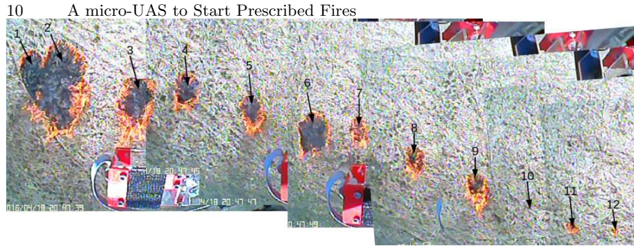
Fig. 9. Video frames from a flyover of the ignition spheres dropped during the fifth flight at Homestead National Monument. Arrows point to locations ignition spheres were dropped.
