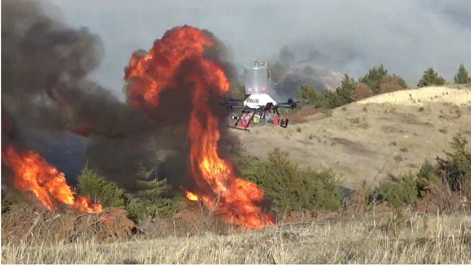
Fig. 1. The prototype UAS-Rx returning after starting a prescribed fire with the Loess Canyon Rangeland Alliance [3].
