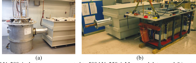
FIGURE 4. (a) 500 kV, 200 A electron gun connected to 500 kV, 250 A Marx modulator; and (b) untanked modulator with the circuit plates visible.
